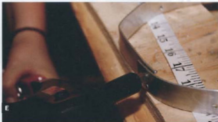
Fig. C: Measure aluminum strip for hanger ring. Fig. D: Mark pilot holes for drilling hanger ring. Fig. E: Rivet (or bolt) ends of ring together.
